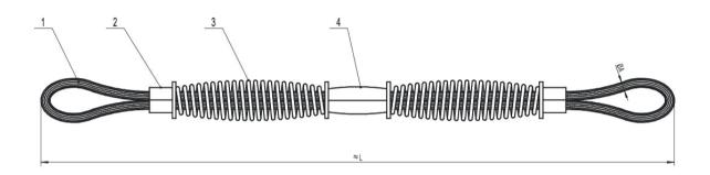
Suitable to prevent injuries or accidents resulting from hose or coupling failure. Safety whip check extends across the hose fittings to give standby safety for hose.
